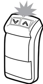
The green light is flashing when the battery is low.
