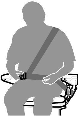
Diagonal side fastening seatbelt
